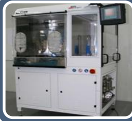
Gläser RiuS Double Extraction Chamber (e.g. to extract particles from automotive parts)
