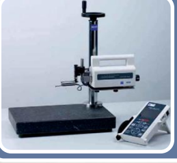
Zeiss SURFCOM FLEX 50A Mobile Control and Analysis Unit for Surfaces (e.g. surface roughness measurement of critical surfaces)
